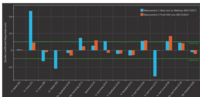
Aberrations of the standard scleral lens (base lens) vs. the wavefront-guided scleral lens (final lens) in the left eye.
