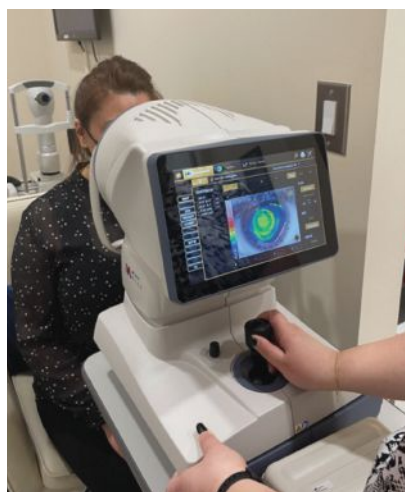
A Topcon Myah in use. The device combines axial length, dry eye testing, meibography and corneal topography in a single machine.
